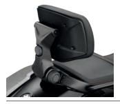
• Dual axis adjustments for the backrest and cushion enable you to dial in comfort and add up to 2" (50 mm) more passenger room.
